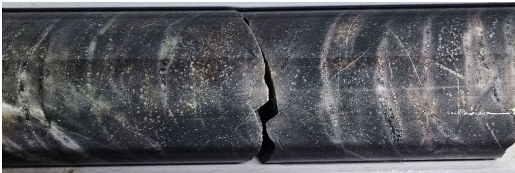
Figure 3: Great Pyramid diamond core (22GPRC014 197.5-200.10m), beneath historic resource area, assay results pending. Intense sheeted quartz-carbonate \pm sulphide veining in strongly silicified, medium to coarse grained sandstones. Historical exploration indicates that veins of this style are cassiterite-bearing and are typical of the mineralised zones.
