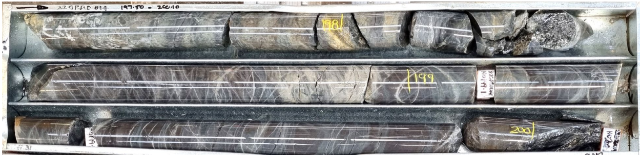
Figure 3: Great Pyramid diamond core (22GPRC014 197.5-200.10m), beneath historic resource area, assay results pending. Intense sheeted quartz-carbonate \pm sulphide veining in strongly silicified, medium to coarse grained sandstones. Historical exploration indicates that veins of this style are cassiterite-bearing and are typical of the mineralised zones.
